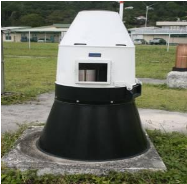
Figure 75: Tilting Siphon Rain Recorder at NMS-Seychelles International Airport
