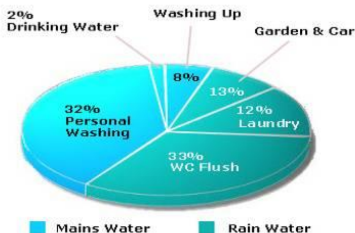
Figure 107: Rain Water Harvesting Contribution to Domestic Needs 6
